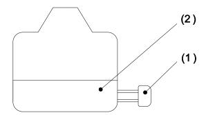
pull off the welding nozzle with an appropriate pair of nippers, slightly turning.
