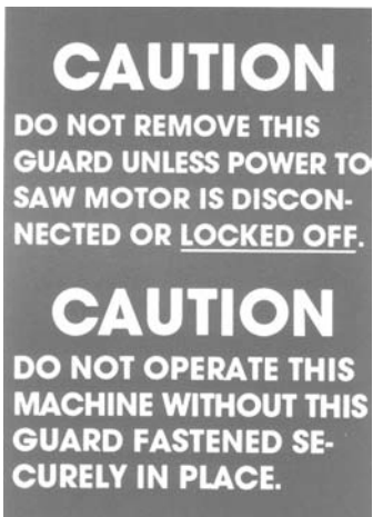
Do Not Remove Blade Guard With Power Connected Do Not Use Without Blade Guard On Machine
