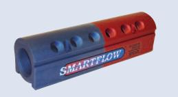
**SWAP® Valves** reduce time required for cooling line evacuation between mold changes to seconds instead of minutes while keeping shop floors clean. SWAP Valves use shop air to evacuate fluid from cooling lines with the single handle motion. The mold can then be changed. Resume main cooling fluid supply with the reverse handle motion.
