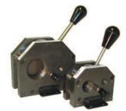
**FasTie® Quick Ejector Tie-In's** slash knockout connection time to seconds with quick couplers and studs. FasTie couplers reside in the press ejector plate. FasTie studs are fastened to each mold in storage. When a mold change is performed, ejector tie in is literally a snap.
