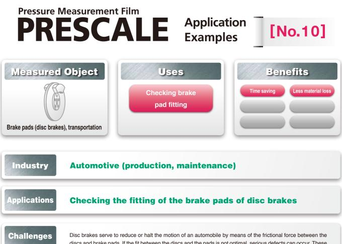
discs and brake pads. If the fit between the discs and the pads is not optimal, serious defects can occur. These include brake failure, uneven component wear, noise and vibration. Thus, the proper fitting of brake pads is important for automobile performance, safety, and part life. Yet, until now, there has been no easy way to check the fit between pads and discs.
