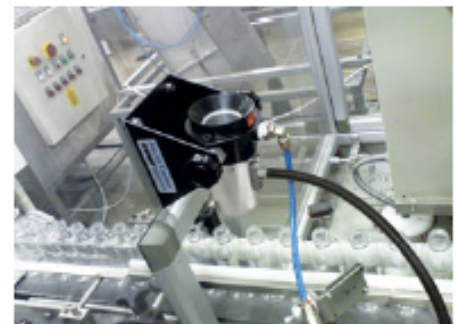
The Model 8292 Ion Air Cannon System eliminates the static and dust prior to filling the bottles.
