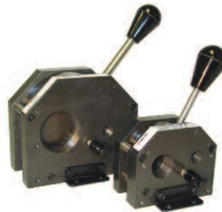
**3 FasTie® Quick Ejector Tie-In's** slash knockout connection time to seconds with quick couplers and studs. FasTie couplers reside in the press ejector plate. FasTie studs are fastened to each mold in storage. When a mold change is performed, ejector tie in is literally a snap.
