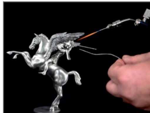
Micro precision soldering of pewter figurine (supplied by Ballantynes Of Walkerburn)
