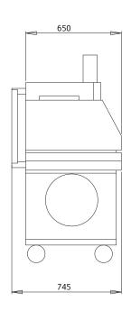
The 911 provides six thermoforming processes in a single machine. A two zone ceramic heater system ensures even heating for vacuum forming and also heats the fan circulated oven. A rotary switch allows the operator to select a process, while a digital timer with audible alarm provides a useful timing guide. Processes available are:
