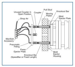
This setup is designed for custom molders who use a variety of injection molds with different knockout patterns and ejector strokes.
