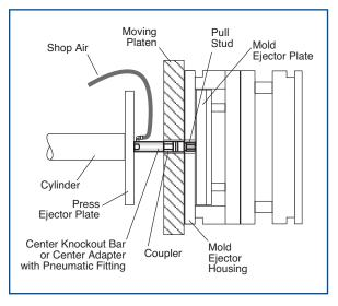
For small presses with a center knockout, replace the cylinder bolt (if present) with a Center Knockout Bar and FasTie coupler.
