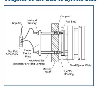
This setup is designed for captive molders, or shops with tools using a standard ejector stroke. Couplers are located at the end of the knockout bars mounted to the press ejector plate.
