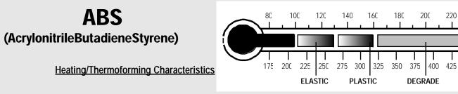
**General** A durable thermoplastic, resistant to weather and some chemicals. It is used in many applications and is particularly popular for vacuum formed components. A limited colour range of black, grey or white is enhanced by the availability of leather grain textures. It is a rigid plastic with rubber like characteristics (Butadiene (its middle component) is also used in the production of synthetic rubbers) which gives it good impact resistance.
