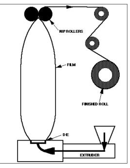
extrudate, through the die and onto the rollers, has been established, air is blown into the tube at the point at which it leaves the die - when it is still pliable - to expand it to the required size. This film tube is flattened, cooled and loaded onto its final reel by the roller system.
