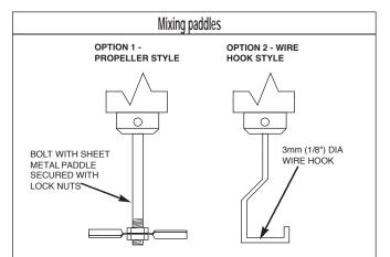
NB: The twists in the paddle blades will act like a propeller, pushing the drill out of the resin. If they have the opposite effect ie. they suck the resin pot onto the paddle, then you should reverse the direction of the drill or turn the paddles over.
