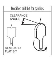
Dimples and hollows can be drilled into the mould using a custom shaped flat drill bit.
