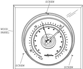
We recommend mounting the read-out on one of our pre-drilled and centered panels.
