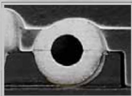
Stripping Area (Round Blades, no wire damage)
