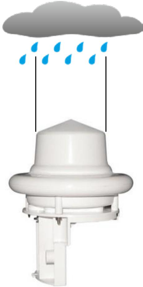
24 GHz Microwave Doppler Radar works with the radar reflection method and measures the precipitation quantity or precipitation intensity by means of the correlation of drop size and velocity.
