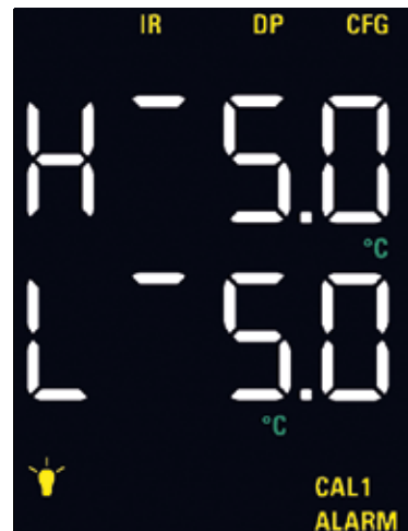
Dew point alarm configuration
