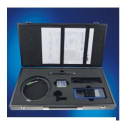
XP201 Order No 5810.20 High Quality Watertight case and Highprecision Temperature/Humidity Sensor Order No 8130.TFF included in delivery.
