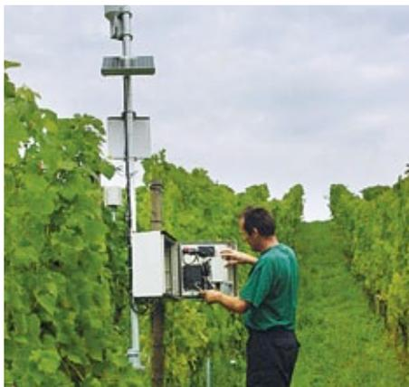
**One external temperature sensor is connectable.**
