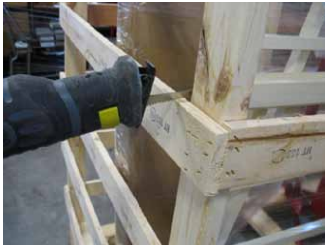
Figure 8: Cutting front/side of wood crate
