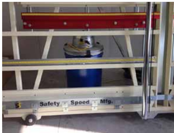
Fig. 62: Midway fence installed
