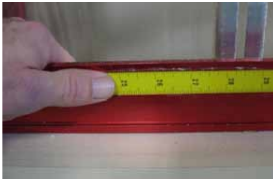
Figure 27: Crosscut Ruler Adjustment
