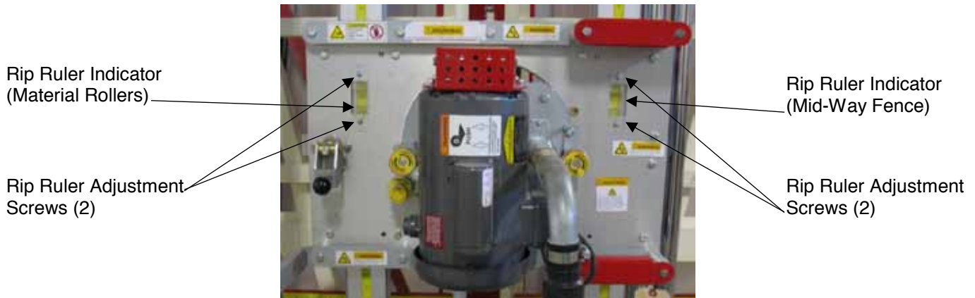
Figure 28: Rip Cut Ruler Adjustment (Rip Position, 7400 shown)
