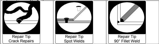
Repair tips are used for crack repairs, filling small holes, spot welding, for reaching tight areas, and for prototyping. Because of their conical shape, the repair tip and prototyping tip offer similar types of welds. Choose the size that best suits your application
