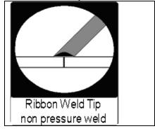
The Ribbon weld tip is used to make a seam weld on thermoplastic materials such as belting and thin sheets. Because this welding tip does not weld down to the root side, it should not be used for regular butt welds.
