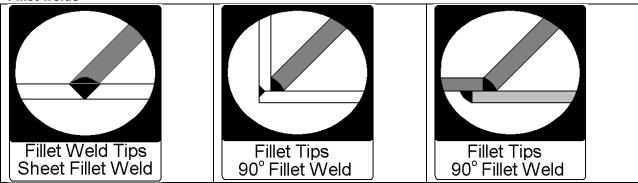
Fillet tips are used mainly for fillet welds [90°] and butt welds. The style of those tips allows one to weld from inside corners out and be able to seal the corners without changing to another tip style. Fillet tips can also be used for crack repairs, as long as the crack is somewhat straight. The longer preheat section allows faster welding speed than welding cracks with the conical tip.
