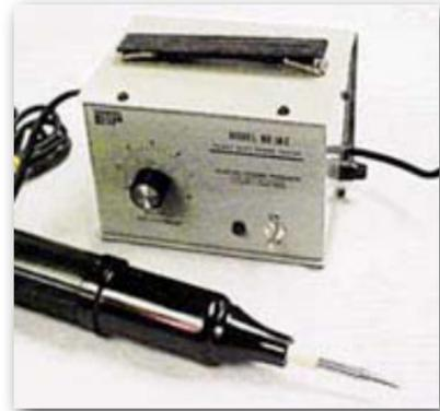
*Defects are detected by electric current grounds through the defect*
