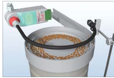
Vibratory bowl feeder (joint nozzle + shower tube)
